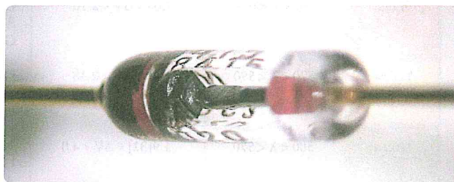
Figure 1-22. 1N914 signal diode used as a radio frequency signal detector.
