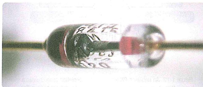
Figure 1-11. A silicon diode, the square crystal silicon can be seen between the two leads.
