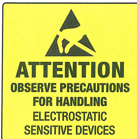
Figure 2-15. Warning sign for an ESD controlled area.
